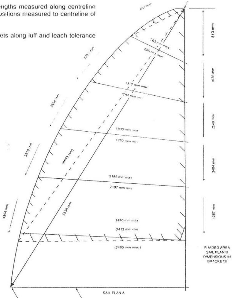
Leech measurement of sail plan A to upper inner edge of boom band and of sail plan B to a point on the upper edge of the boom 2490mm from the aft side of the mast at the lower band.
