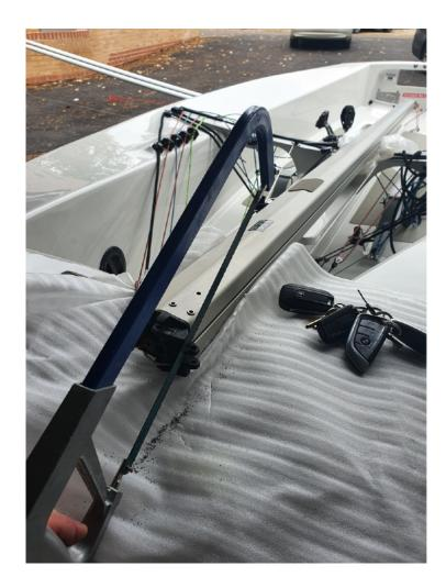
To check the mast foot position fix a tape measure to the forward face of your mast and measure to distance to the transom flap cutout.
