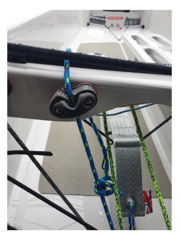
On the standard Winder centreboard uphaul/ downhaul system I have fitted a larger diameter rope for ease of handling.
