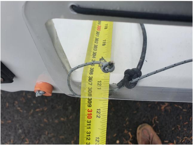
Check for mast wobble(!) in the gate. If required, use your partners credit card to slide under the mast packer and tape it in place to stop it coming out. Pack both sides equally to keep the mast central.
