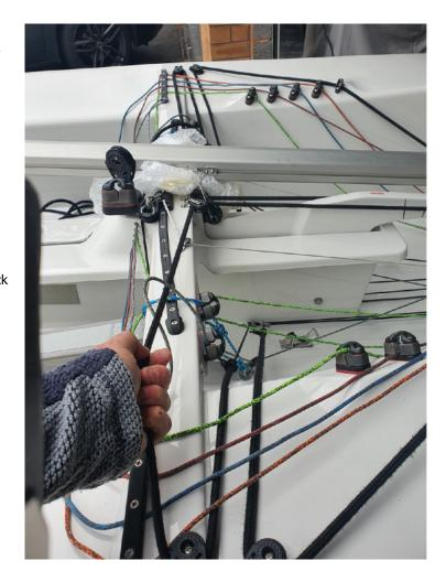
On the inboard end of the boom I cut off the plastic lugs which would normally take the tack pin. On a North sail especially, these can get in the way when pulling on the inhaul and cunningham in a breeze.
