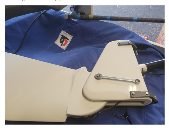
I feed the toestrap adjustment rope around the thwart and tie it back onto itself so there is less chance of the rope coming out the cleat. This also tidies up the rope tails in this area so you have less issues with tangles and/or grabbing the wrong control line in the heat of battle.
